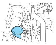
Only use a washer fluid that meets Ford specifications. Do not use any special washer fluid such as windshield water repellent type fluid or bug wash. They may cause squeaking, chatter noise, streaking and smearing. Refer to the *Maintenance product specifications and capacities* section in this chapter.
